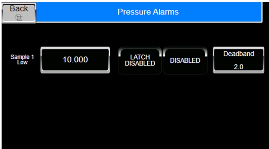
Each of the concentration alarms on this screen are set by pressing the desired alarm value button, entering the new alarm value in the pop-up window, pressing enter to return to this screen. The alarm is then enabled by pressing the DISABLED/ENABLED button. Each alarm by default is a momentary alarm, but each can be changed to a latched alarm by pressing the LATCH DISABLED/ENABLED button. Note that only one concentration alarm is standard, the additional concentration alarms are optional.
